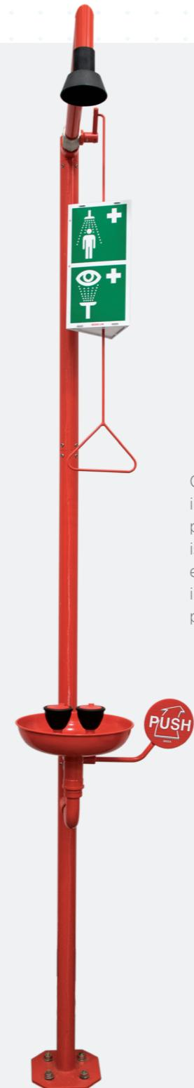
Combined Eye wash and Body showers are designed and intended to be installed in close range of persons working in a potentially hazardous area. The main purpose of these devices is to immediately deliver a flushing fluid in a sufficient volume to extinguish flames and/or to flush the body following exposure to injurious substances or heat. With this accomplished the injured person can proceed to medical care.
